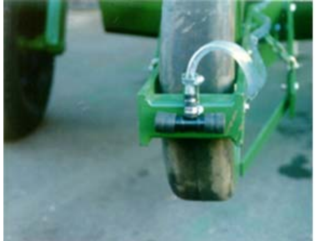
Detergent applicator for non-wetting soil.
