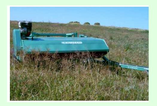
The Kimseed Brush Harvester provides a simple and effective means of collecting grass seeds. As the harvester moves through the seeding grasses, ripened seed is combed upwards off the plants and thrown rearwards into a catchment hopper. The seed collected by the Harvester is relatively clean and requires minimal cleaning or processing and is therefore more cost effective.
