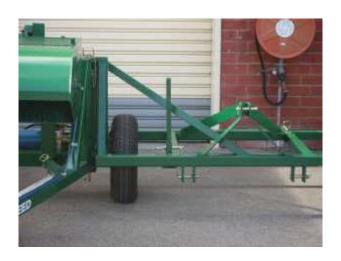
Remove the drawbar only when the weight box counterbalance has been filled with sand or rocks or concrete slabs.
