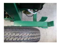
Connect the 3 Point linkage attachment to the tractor linkage.
