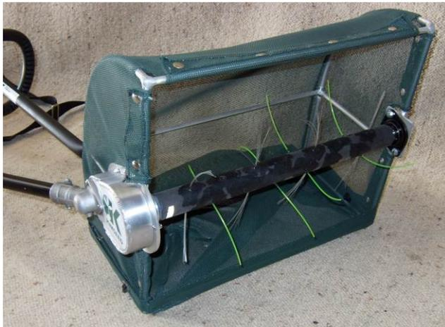
**A special lightweight brush drive assembly allows for lower brush speed and more control in collecting ripened seed and leaving green seed.**
